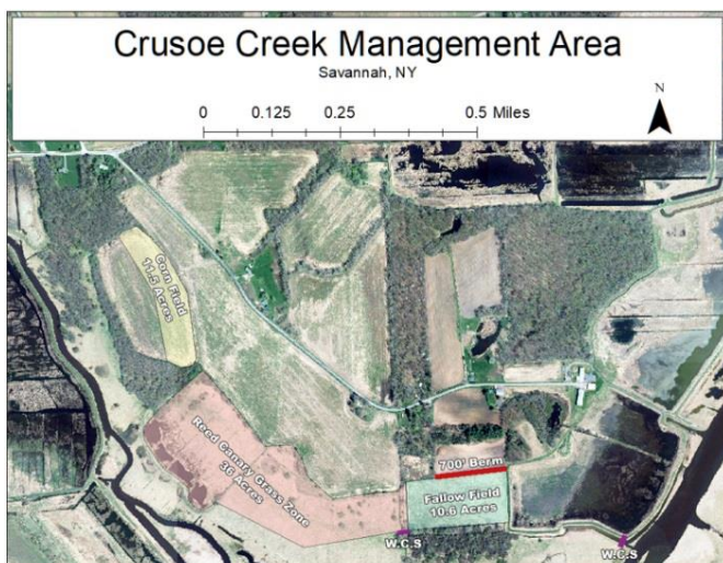
Figure 1. Map of the Crusoe Creek management area, including the three management areas, berm along private farm field to prevent flooding and proposed water control structure (WCS) placement.
